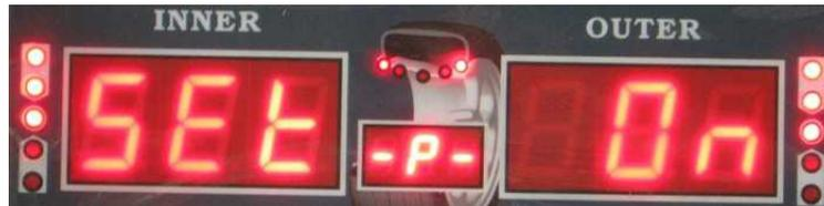
To Change this setting to off, push the **UP** or **DOWN** arrow. Once you have the setting correct to fit your needs, press the **ENTER** button to return to the system settings main menu. You can now use the **UP** or **DOWN** arrows to move to the next setting you wish to change.
