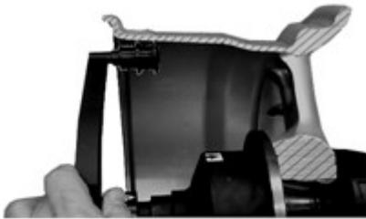
In ALUS mode, pull the gauge against the chosen correction plane on the inside of the rim, press
